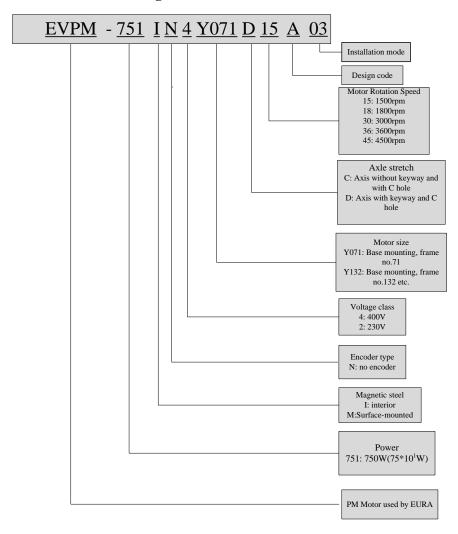
Fig 1-2 PM Motor naming rule
