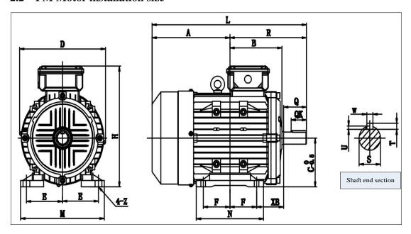
Fig 2-1 PM Motor IMB3 Installation Structure
