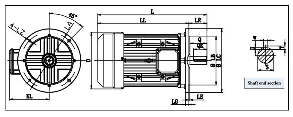
Fig 2-2 PM Motor IMB5 installation structure
