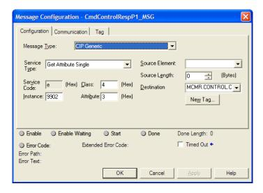
A 5-word response will be passed back through the MSG instruction to the controller tag array, MCMR.CONTROL.CMDCONTROLP1.CMDCONTROLRESP or MCMR.CONTROL.CMDCONTROLP1.CMDCONTROLRESP, depending on whether the Event Command was sent for Port 1 (9901) or Port 2 (9911). The following table lists the 5-word response data received.
