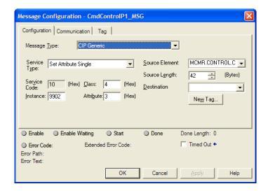
Status Data can be returned to the processor using a "Get Attribute Single" service type MSG instruction. If you follow the provided sample ladder logic or use the provided Add-On Instruction (AOI), the *Get Command Control Status* MSG will be triggered at the same time as the *Send Command Control* message by the same controller tag, MCMR.CONTROL.CMDCONTROLP1.CMDTRIGGER for Port 1 or MCMR.CONTROL.CMDCONTROLP2CMDTRIGGER for Port 2.
