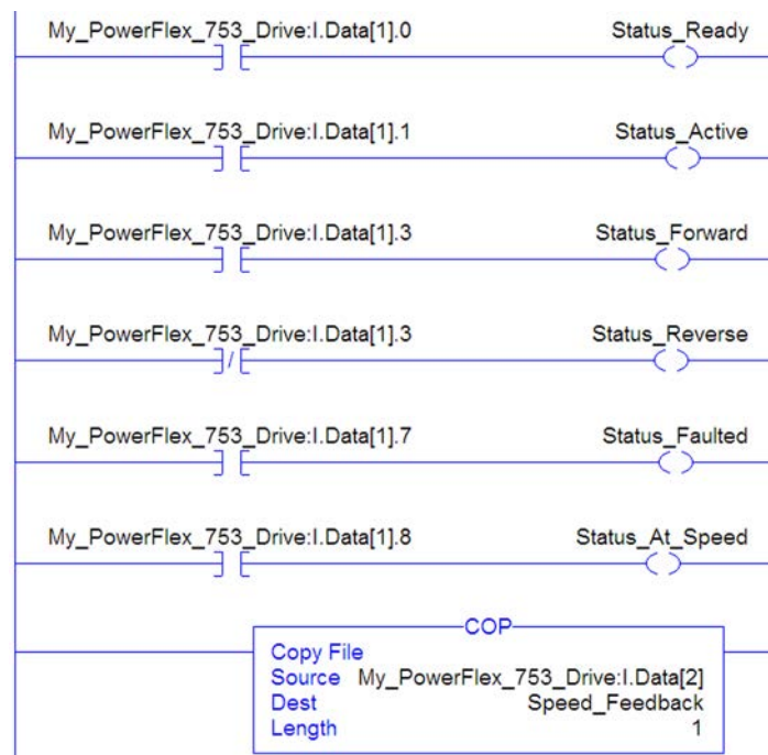
Figure 20 - ControlLogix Controller Example Ladder Logic Program Using a Drive Generic Profile for Logic Status/Feedback
