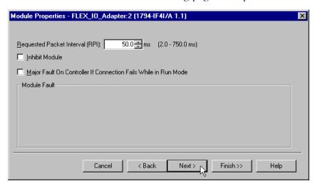
**5.** This window allows you to adjust the **Requested Packet Interval (RPI)** to meet your system's requirements. For this example you can leave it at the default 50 ms rate shown above. This RPI will be used for the direct connection to this analog module. The two rack connected digital I/O modules will continue to communicate at the RPI of the rack connection.
