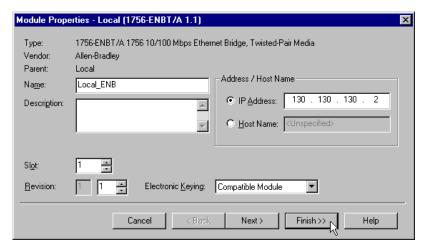
**4.** Enter or select the following parameters: **Name**, **IP Address**, **Slot**, and **Electronic Keying**. We used the following values:
