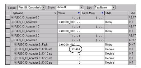
**4.** Monitor channel 0 of the 1794-IF41/A input module (FLEX\_IO\_Adapter:2.I.Ch0Data above). You should see the value slowly rise to approximately 32000, reset to zero, start rising again, etc., as the output of the timer is received from the 1794-OF41/A output module.
