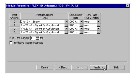
**8.** Use the pull-down list to set the **Voltage/Current Range** for **Channel 0** to "0 to 10V - Binary". (This range allows you to easily monitor the output with a voltmeter when you test the application.)
