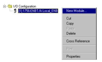
**1.** In the Project window, right click on the local 1756-ENBT module under the I/O Configuration folder and select **New Module** from the pop-up window. The **Select Module Type** window will open.
