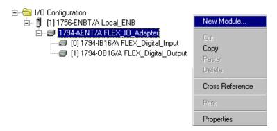
Right click on the 1794-AENT adapter under the I/O Configuration folder and select New Module from the pop-up window. The Select Module Type window will open.
