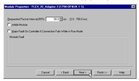
**5.** This window allows you to adjust the **Requested Packet Interval (RPI)** to meet your system's requirements. For this example you can leave it at the default 50ms rate shown above. This RPI will be used for the direct connection to this analog module. The other analog module will communicate at the RPI selected for its connection. The two rack connected digital I/O modules will continue to communicate at the RPI of their rack connection.
