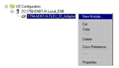
**1.** Right click on the remote **1794-AENT** adapter under the I/O Configuration folder and select **New Module**.
