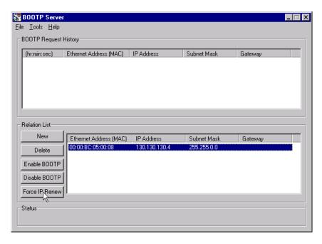
**5.** Select the device from the **Relation Lis**t and click on the **Force IP Renew** button. Then cycle power to the device.
