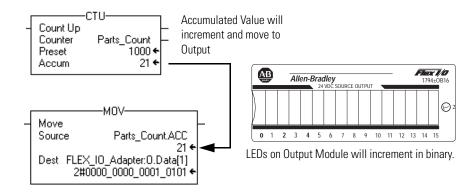
**5.** Press and release the momentary switch at Input 2 (Reset) on the 1794-IB16 input module. You should see the accumulated value of the Parts\_Count reset to zero and all of the LEDs on the 1794-OB16 output module turn off.
