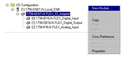
Right click on the 1794-AENT adapter under the I/O Configuration folder and select New Module from the pop-up window. The Select Module Type window will open.
