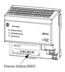
Before you can use your 1794-AENT adapter, you must configure its IP address, and optionally, its subnet mask and gateway address. You can use the Rockwell BootP utility to perform the configuration. You can also use generic BootP software or, within some limitations, a DHCP server.
