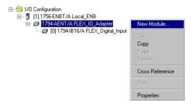
**6.** Right click on the **1794-AENT** adapter and again select **New Module**. The **Select Module Type** window will open.
